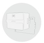
2 Hang and secure AC Battery to mounting bracket.
